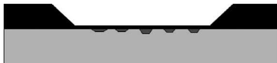
Fig. 1. Schematic side view of zircons (dark gray) embedded in epoxy (light gray), for X-PEEM analysis (not to scale). The region to be imaged (center) is sputter-coated with 10 Å Pt/Pd (black). Electrical contact is made at the edges, where the Pt/Pd coating is 500 Å thick.
