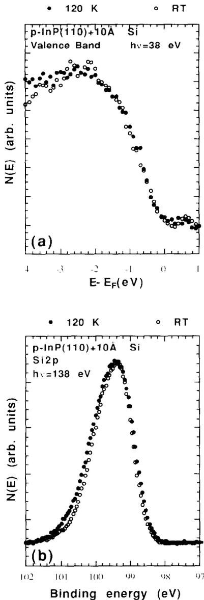
Fig. 4. Valence band (a) and Si2p (b) photoemission spectra of Si/p-InP heterojunction taken at RT – open circles – and LT – full circles –.
