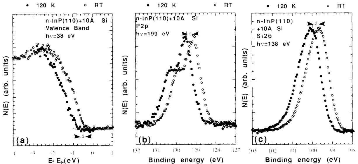
Fig. 3. Valence band (a), P2p (b) and Si2p (c) spectra of Si/n-InP heterojunction obtained at room temperature (RT) – open circles – and at 120 K (LT) – full circles –. At low temperature there is a rigid shift of 0.3 eV to higher binding energies of all the spectral features.
