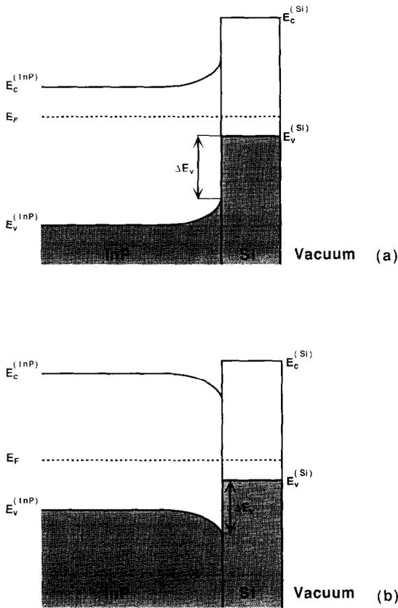
Fig. 1. Band structure of the Si/n-InP(110) (a) and Si/p-InP(110) (b) interfaces. At equilibrium the Fermi levels of InP and Si are aligned, and the InP bands are bent in opposite ways in the two cases. The  $x$  axis is not in scale, i.e., the InP depletion layer is more than 100 Å wide, while the Si layer is 10 Å thick. The band discontinuity  $\Delta E_v$  (0.6–0.7 eV) is shown in the figures.
