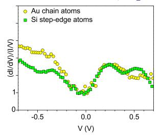
**Figure 3.** Normalized STS (dI/dV)/(I/V) spectra taken at room temperature on the edge of the graphitic Si strip and the Au chain at the center of the terrace, see figure 2(a). The peak at +0.5 V exists only at the step edge.
