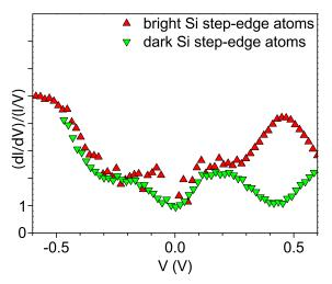
**Figure 4.** Normalized STS (dI/dV)/(I/V) spectra taken at 40 K on the bright and dark Si step-edge atoms, see figure 2(b). A clear difference is evident in the unoccupied states, for which the bright atoms exhibit a strong peak at 0.5 eV not seen on the dark atoms. This peak is in excellent agreement with the predicted unoccupied minority-spin state of the spin-polarized Si atoms, shown in figure 1(b).
